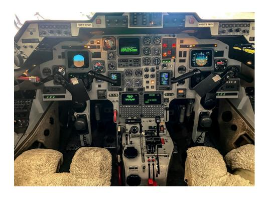
**Flight Directors** Honeywell SPZ-8000 **Autopilot** Honeywell DFZ-800 Radar Honeywell Primus 800 Comm Dual Honeywell RCZ-833 Nav Dual Honeywell DM-850 DME Dual Honeywell RCZ-833 **ADF** Dual Honeywell RCZ-833 **Transponders** Dual Garmin GTX 3000 Radar Altimeter Honeywell RT-300
